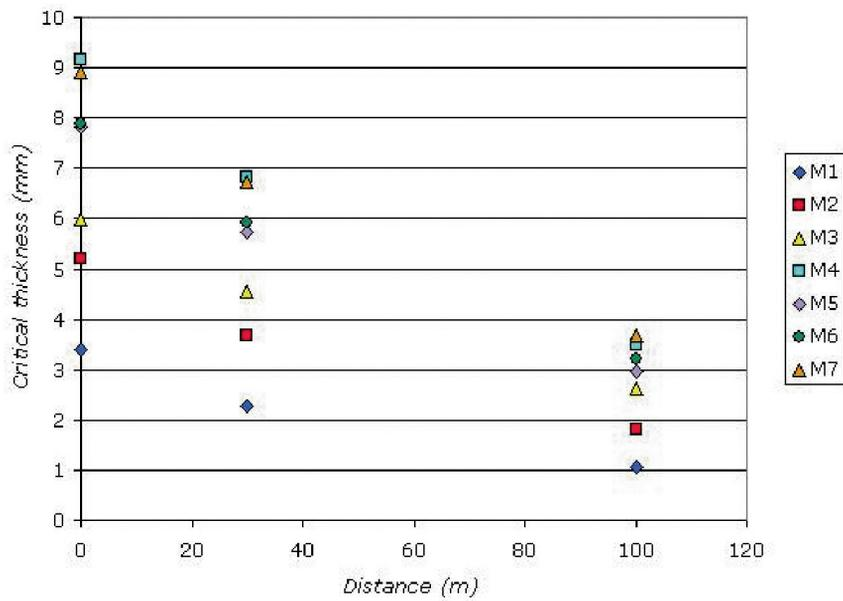
Fig. 3 Critical thickness of armour at variable distances for different 17th-century muskets based on test-firing experiments [Krenn, 1991]; for weapon acronyms (M1-7), see Table 1.
