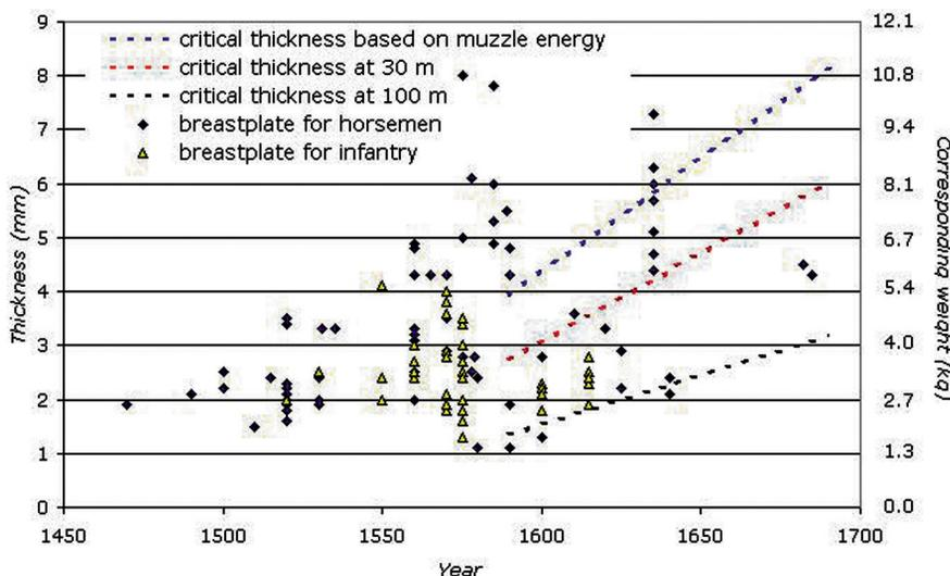
Fig. 4 Critical musket-proof thickness of armour over time; armour thickness measured by Williams et al. (see notes 17-18)
