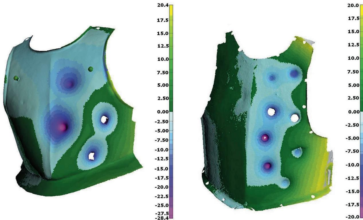
Fig. 2 3D laser scan showing the profile of breastplates after ballistic testing
