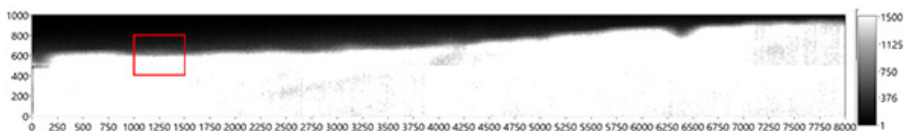
Figure 12. Cu peak-area mapping of a cross-section of etched test plate G. The area in the red square can be seen in greater detail in Figure 13.
