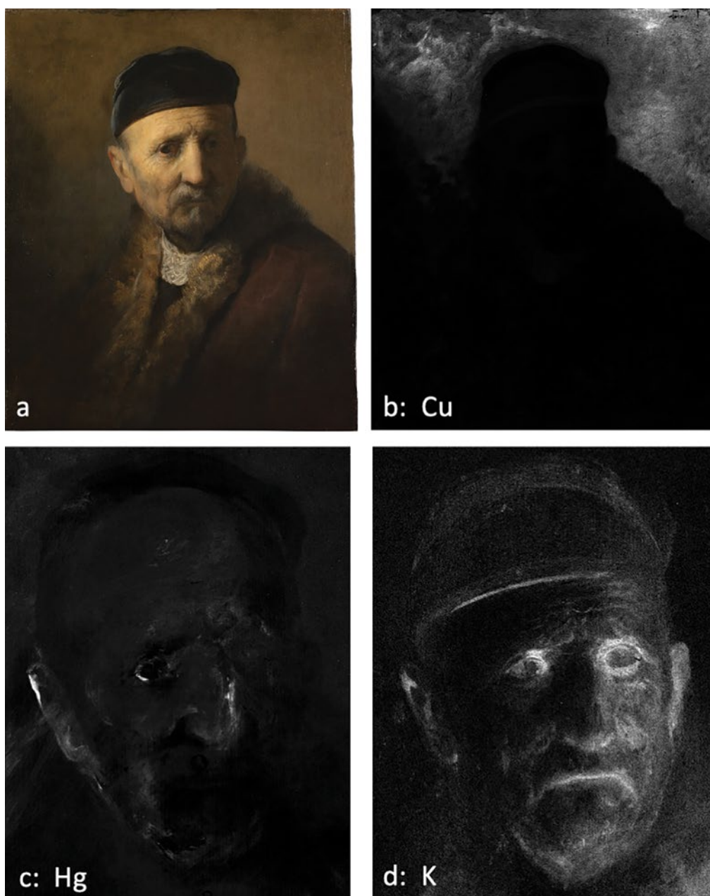
Figure 4 Rembrandt (?), Tronie of an Old Man , c.1630–31, oil on panel, 46.9 × 38.8 cm, Mauritshuis, The Hague, inv. no. 565: (a) recto; (b) MA-XRF map for copper (Cu-K); (c) mercury (Hg-L); (d) potassium (K-K). © Mauritshuis, The Hague.
