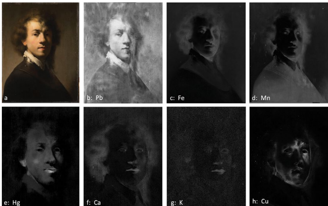
Figure 3 Rembrandt (studio copy), Portrait of Rembrandt with a Gorget , 1629, oil on panel, 37.9 × 28.9 cm, Mauritshuis, The Hague, inv. no. 148: (a) recto; MA-XRF maps for (b) lead (Pb-L), (c) iron (Fe-K), (d) manganese (Mn-K), (e) mercury (Hg-L), (f) calcium (Ca-K), (g) potassium (K-K) and (h) copper (Cu-K). © Mauritshuis, The Hague.
