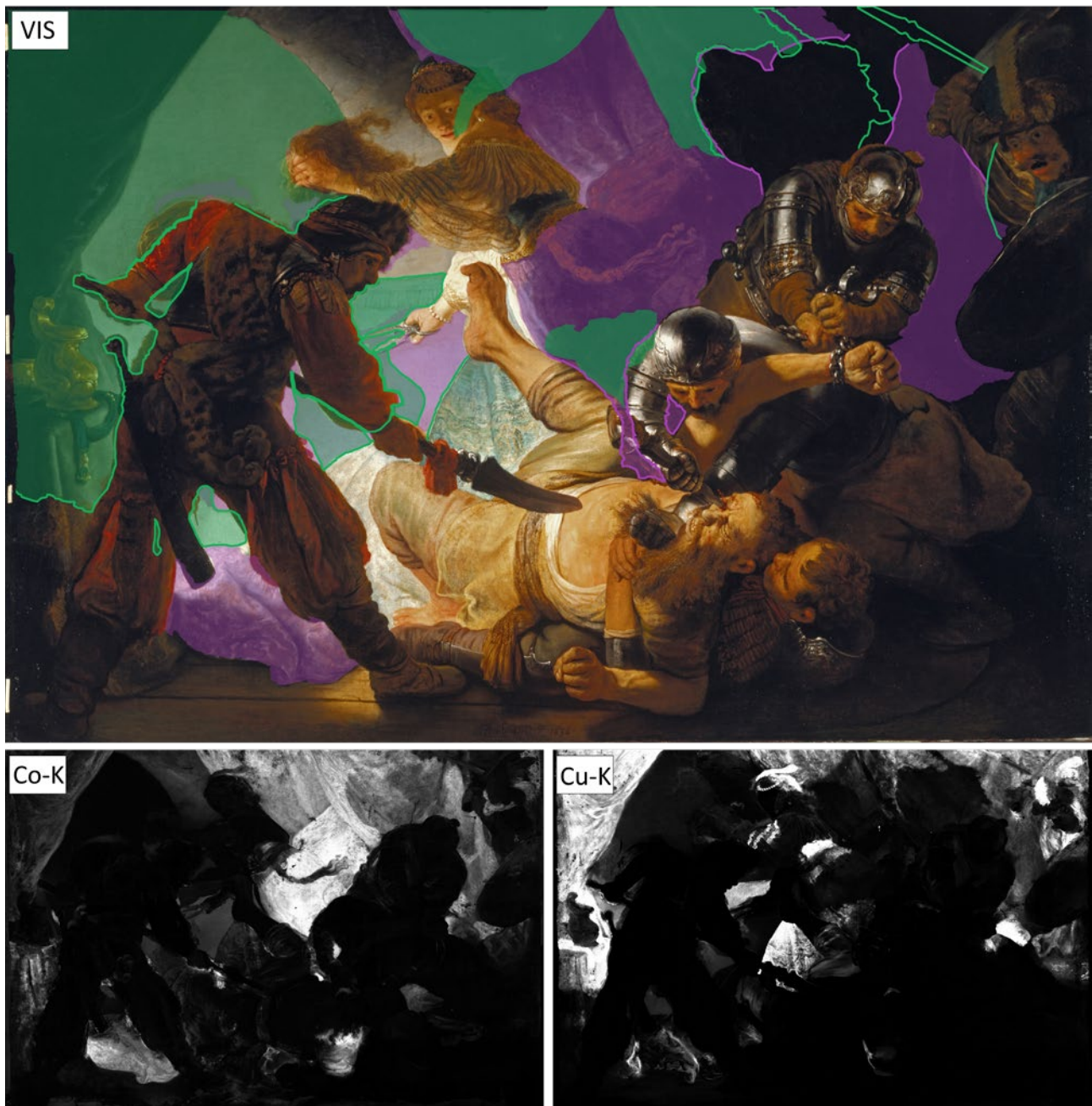
Figure 4 Mapping of the two blue underpaintings (VIS) and micro-XRF elemental distribution images of cobalt (Co-K) and copper (Cu-K). In addition to the light-toned and brown underpaintings, the detected blue underpaintings with smalt (Co-K) and a copper blue (Cu-K) also played an important part in establishing the composition. © Städel Museum, Frankfurt am Main (images: Mareike Gerken).
